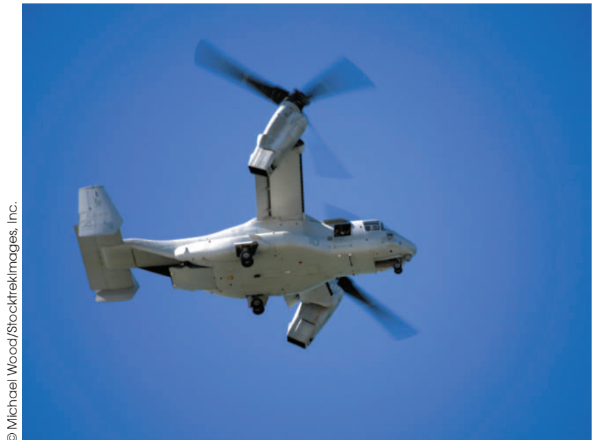
The engine/propeller units at the wingtips of this aircraft can tilt from a vertical takeoff position to a horizontal position for forward flight.
