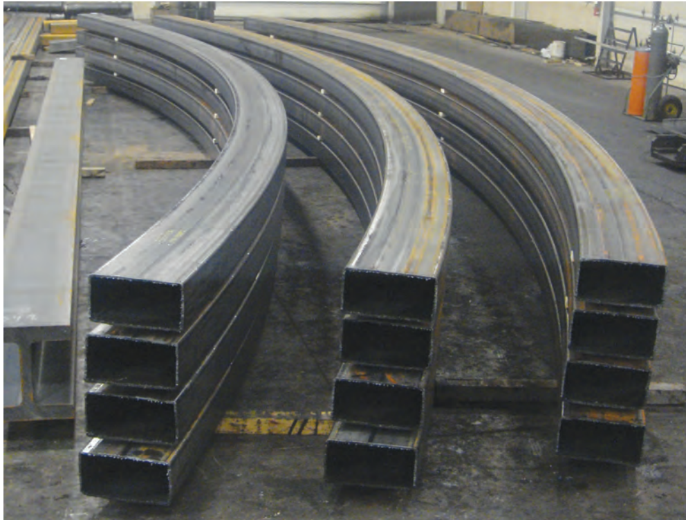
(a) Rectangular HSS bent the hard way
