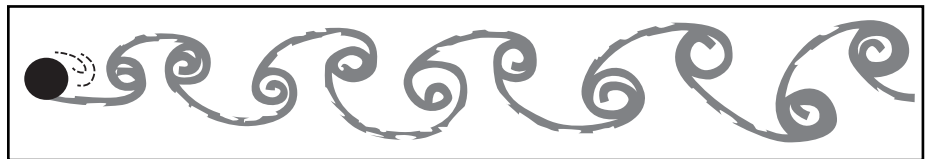
Figure 9.1 2D schematic representation of vortices generated in the wake of a cylinder.
