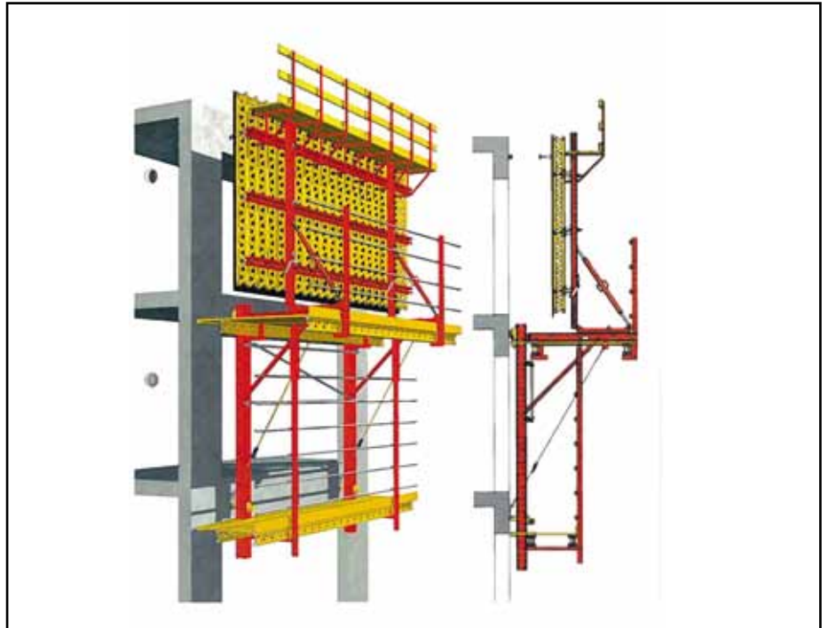
Figure 6.3 An example of a crane-lifted jump-form. Image: Peri Ltd.
