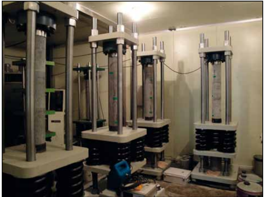
Figure 11.4 Measuring creep strain from concrete specimens in a climate chamber.
