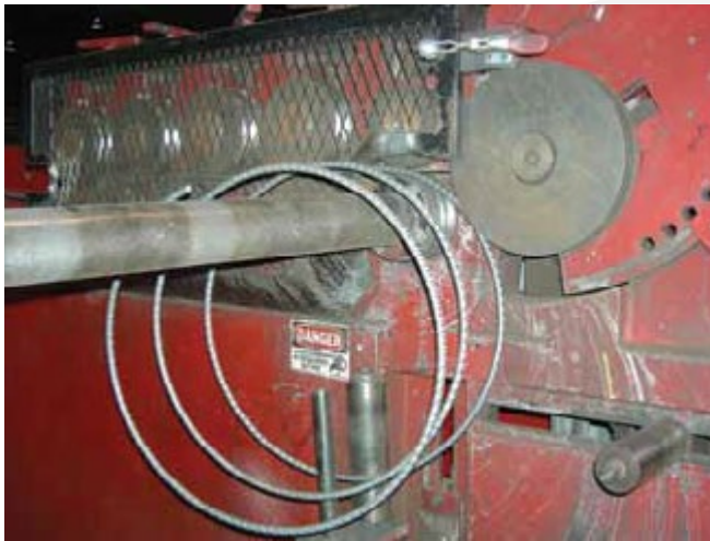
Fig. 7: Fabrication of a continuously wound circular tie or spiral on a “spiral machine”
