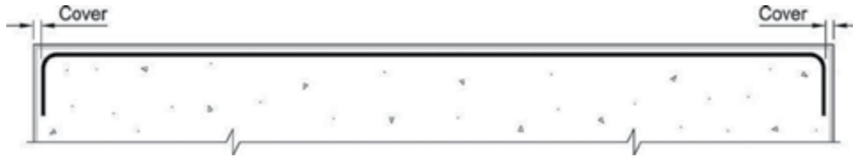
Fig. 3.2.7a—Single bar with hook at both ends.
