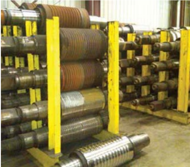
Fig. RFI 12-02.1: Examples of finish (or final) rolls used on a reinforcing bar line to roll in the deformations and bar marks. Several of the rolls are kept in inventory at the steel mill (Photo courtesy of Nucor Steel, Marion, OH)
