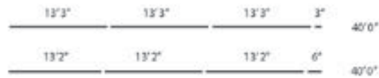
Fig. 3: Routine shortcutting of bars often just results in more crop bar, rather than an actual saving of steel
