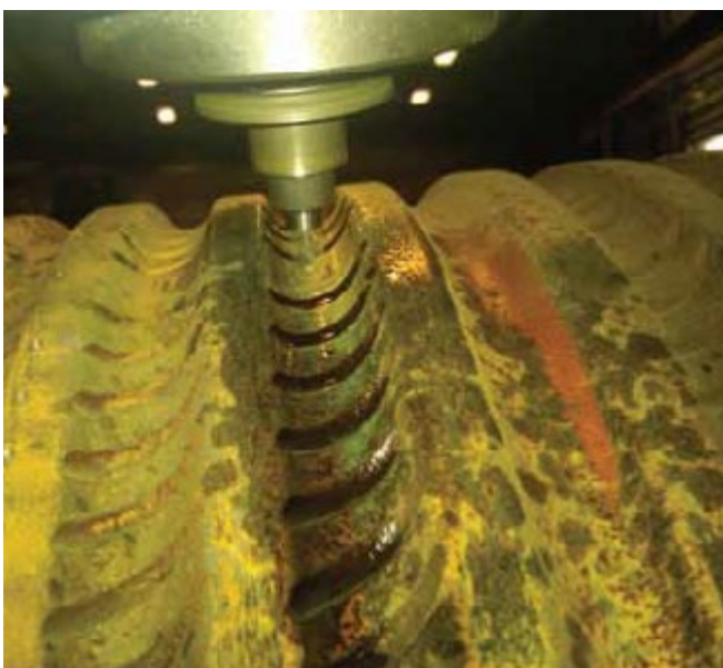
Fig. RFI 12-02.2: A four-axis milling machine is used to re-cut and provide better definition to the deformations on a worn roll surface (Photo courtesy of Nucor Steel, Marion, OH)
