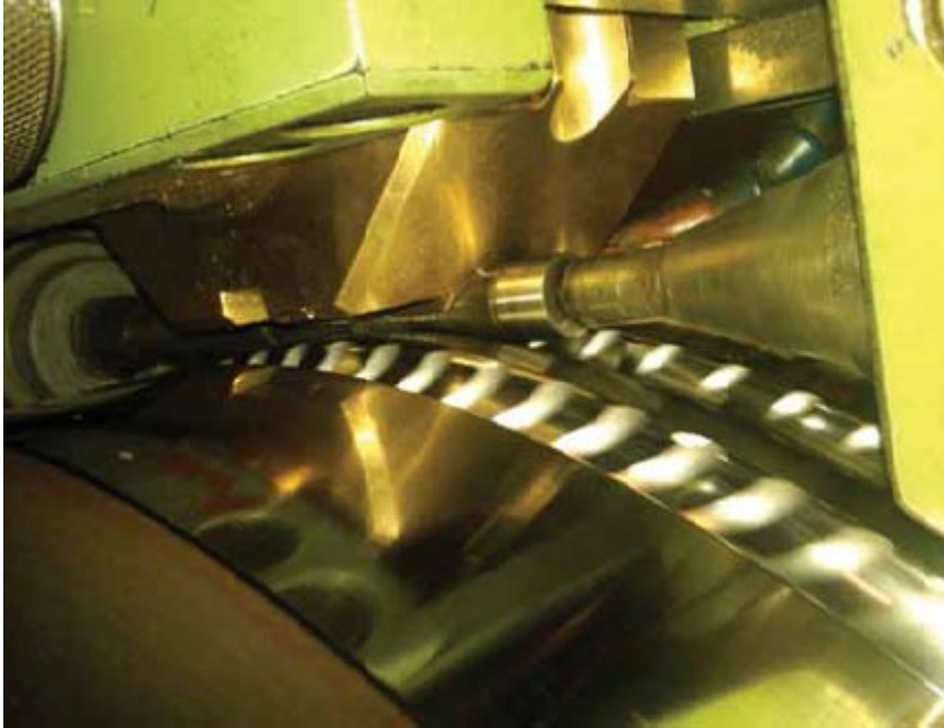
Fig. RFI 12-02.3: The roundness of the slot is also re-established in the milling machine. The roll surface is then cleaned and polished to provide a smooth surface free of burrs and filings, so the roll produces a sharp deformation on the reinforcing bar stock (Photo courtesy of Nucor Steel, Marion, OH)
