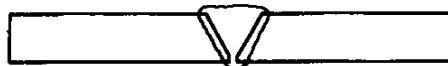
QW-463.1(b) PLATES — 3/4 in. AND OVER THICKNESS AND ALTERNATE FROM 3/8 in. BUT LESS THAN 3/4 in. THICKNESS PROCEDURE QUALIFICATION
