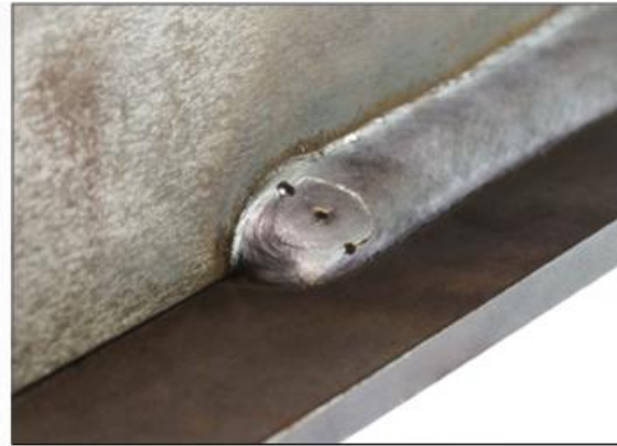
With crater filling - perfect end of weld seam
