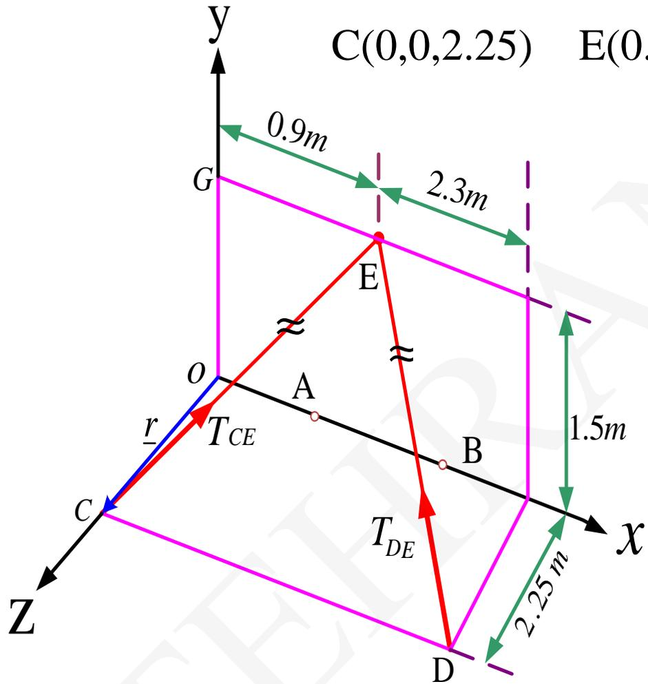
$$C(0,0,2.25) \quad E(0.9, 1.5, 0) \quad \underline{T}_{CE} = T_{CE} \underline{\lambda}_{CE}$$
