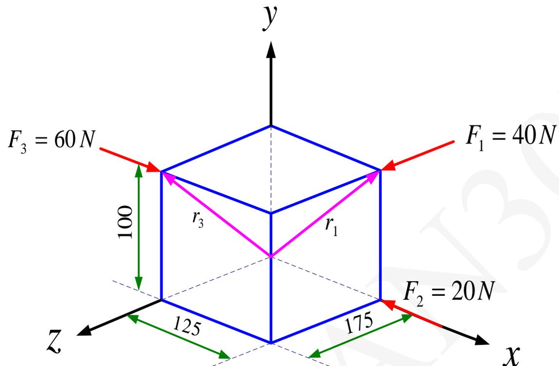
$$\underline{M}_2 = 0 \quad \underline{F}_3 = 60 \underline{i} \quad \underline{r}_3 = 0.1 \underline{j} + 0.175 \underline{k}$$
