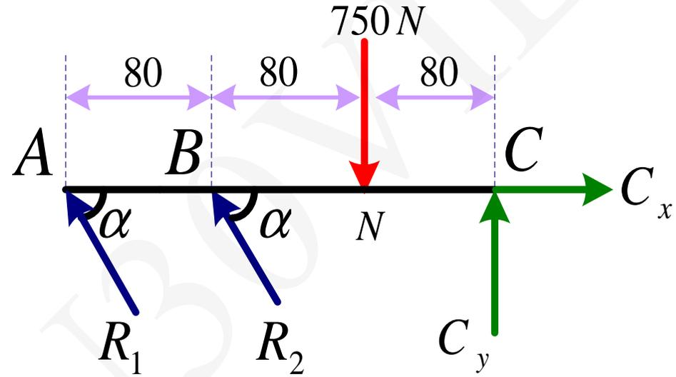
$$\sum M_C = 0 \Rightarrow R_1 \sin \alpha \times (0.24) + R_2 \sin \alpha \times (0.16) - 750 \times 0.08 = 0$$
