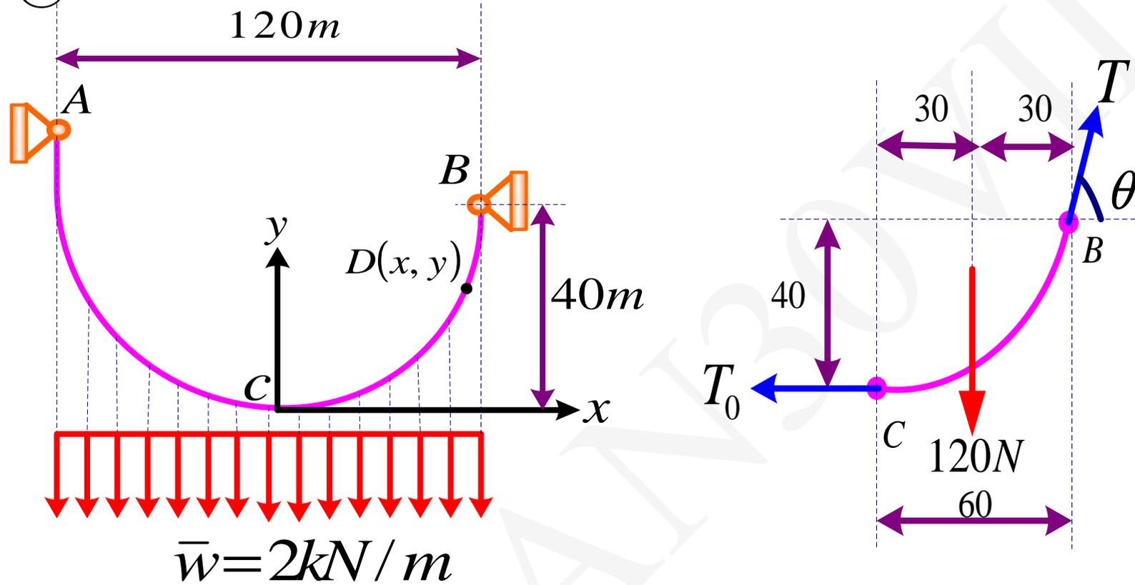
$$S_{CB} = x_B \left[ 1 + \frac{2}{3} \left( \frac{y_B}{x_B} \right)^2 - \frac{2}{5} \left( \frac{y_B}{x_B} \right)^4 + \frac{4}{7} \left( \frac{y_B}{x_B} \right)^6 \right] \dots$$
