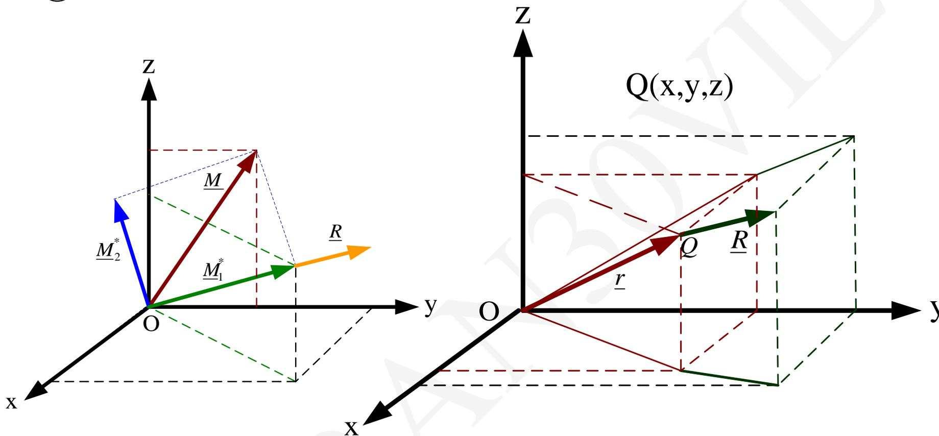
$$\underline{R} = F_1 \underline{i} + F_2 \underline{j} + F_3 \underline{k}$$
