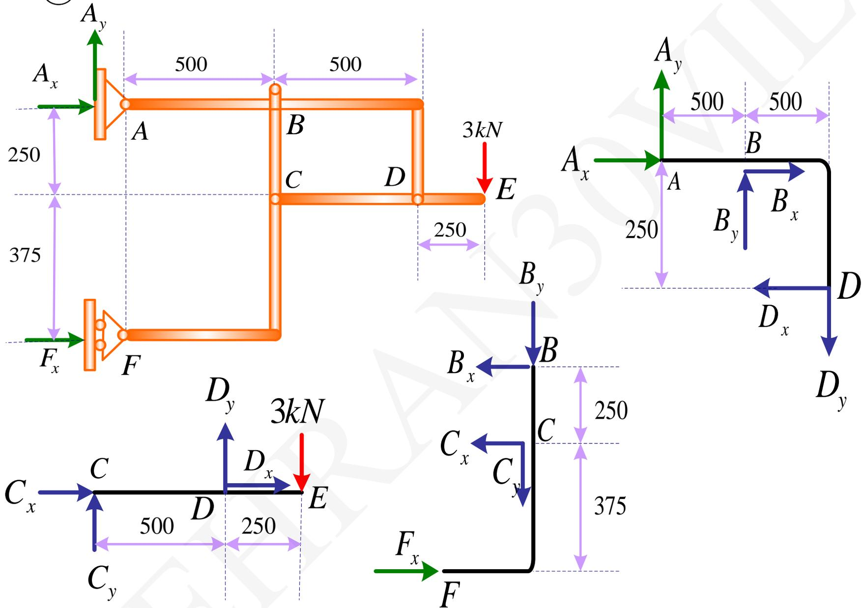
$$A_x = -6kN \quad F_x = 6kN \quad A_y = 3kN$$
