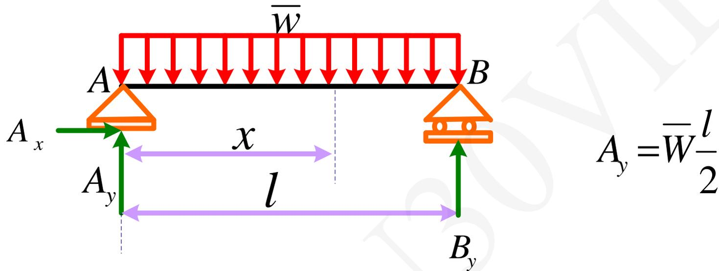
$$\frac{dV}{dx} = -\bar{W} \Rightarrow dV = -\bar{W} dx \Rightarrow \int_{A_y}^V dV = -\bar{W} \int_0^x dx$$
