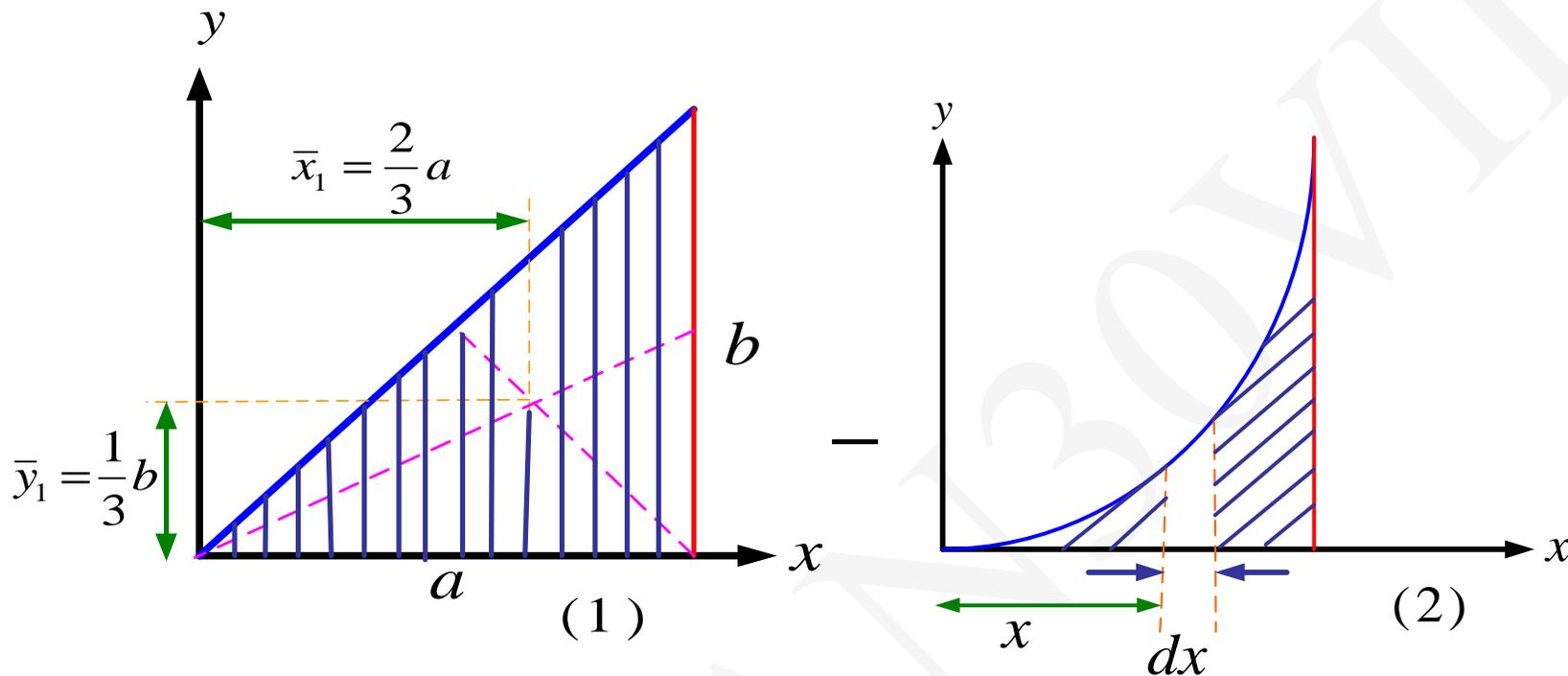
$$\int x dA = \int x_{el} dA = \int xy dx = \frac{b}{a^3} \int_0^a x^4 dx = \frac{b}{a^3} \left( \frac{1}{5} \right) a^5 = \frac{1}{5} a^2 b$$
