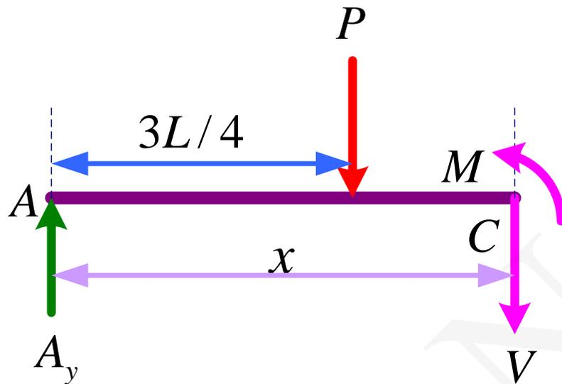
$$\left. \begin{aligned} \sum F_y = 0 &\Rightarrow A_y - P - v = 0 \Rightarrow v = \frac{-3P}{4} \\ \sum M_C = 0 &\Rightarrow A_y x - \left(x - \frac{3L}{4}\right) P - M = 0 \Rightarrow M = \frac{3P}{4}(l - x) \end{aligned} \right\} 3L/4 \leq x \leq L$$
