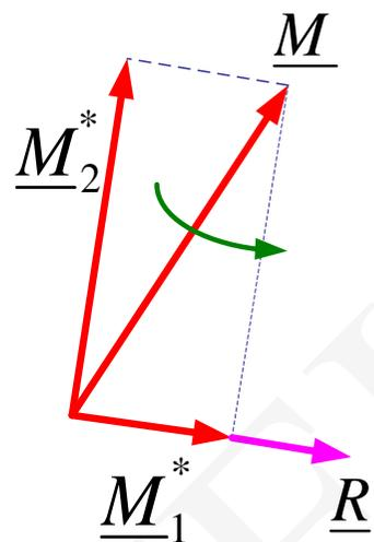
$$\underline{\lambda} = \frac{\underline{R}}{|\underline{R}|} = \frac{40(\underline{i} + \underline{k})}{40\sqrt{2}} = \frac{\sqrt{2}}{2}(\underline{i} + \underline{k})$$
