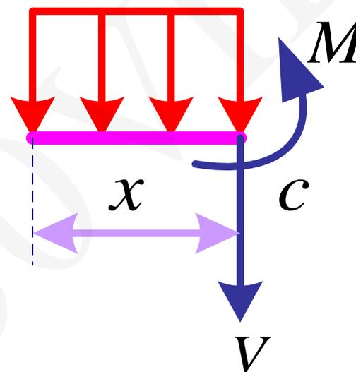
$$\left. \begin{aligned} \sum F_y = 0 &\Rightarrow \bar{W}x + v = 0 \Rightarrow v = -\bar{W}x \\ \sum M_c = 0 &\Rightarrow \bar{W}x\left(\frac{x}{2}\right) + M = 0 \Rightarrow M = -\frac{Wx^2}{2} \end{aligned} \right\} 0 \leq x \leq l/4$$
