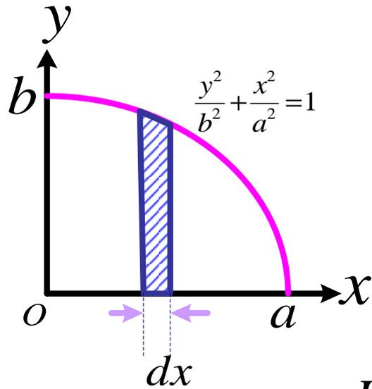
$$\int \bar{x}_{el} dA = \int xy dx = b \int_0^a x \sqrt{1 - \frac{x^2}{a^2}} dx = \frac{ba^2}{3}$$
