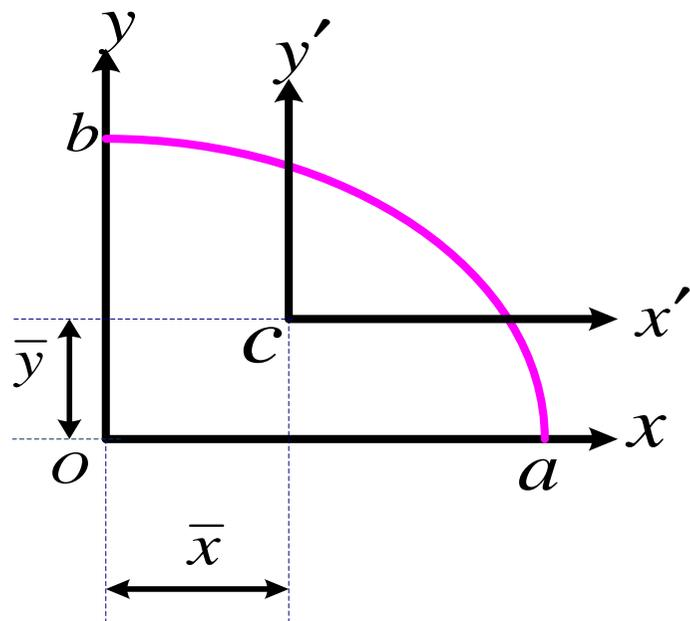
$$I_{xy} = I_{x'y'} + \bar{x}\bar{y}A$$
