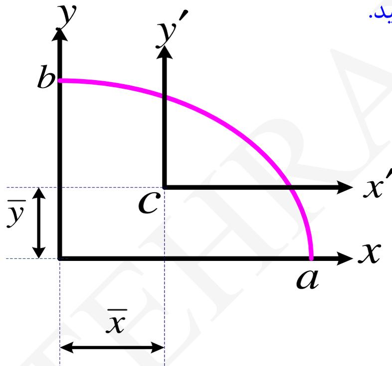
$$\begin{cases} I_{x'} = 1097.6 \text{mm}^4 \\ I_{y'} = 4390.4 \text{mm}^4 \\ I_{x'y'} = -658.8 \text{mm}^4 \end{cases}$$
