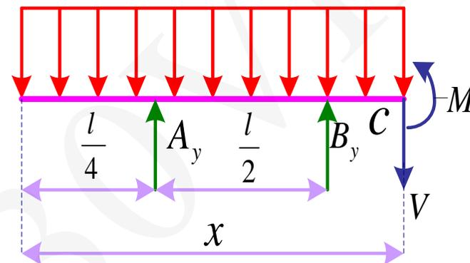
$$\left. \begin{aligned} \sum F_y = 0 &\Rightarrow A_y + B_y - \bar{W}x - v = 0 \Rightarrow v = \bar{W}(l - x) \\ \sum M_C = 0 &\Rightarrow -A_y \left( x - \frac{l}{4} \right) + \bar{W}x \left( \frac{x}{2} \right) - B_y \left( x - \frac{3l}{4} \right) + M = 0 \\ &\Rightarrow M = \frac{\bar{W}l}{2} \left( x - \frac{l}{4} \right) + \frac{\bar{W}l}{2} \left( x - \frac{3l}{4} \right) - \frac{\bar{W}x^2}{2} \end{aligned} \right\} \frac{3l}{4} \leq x \leq l$$
