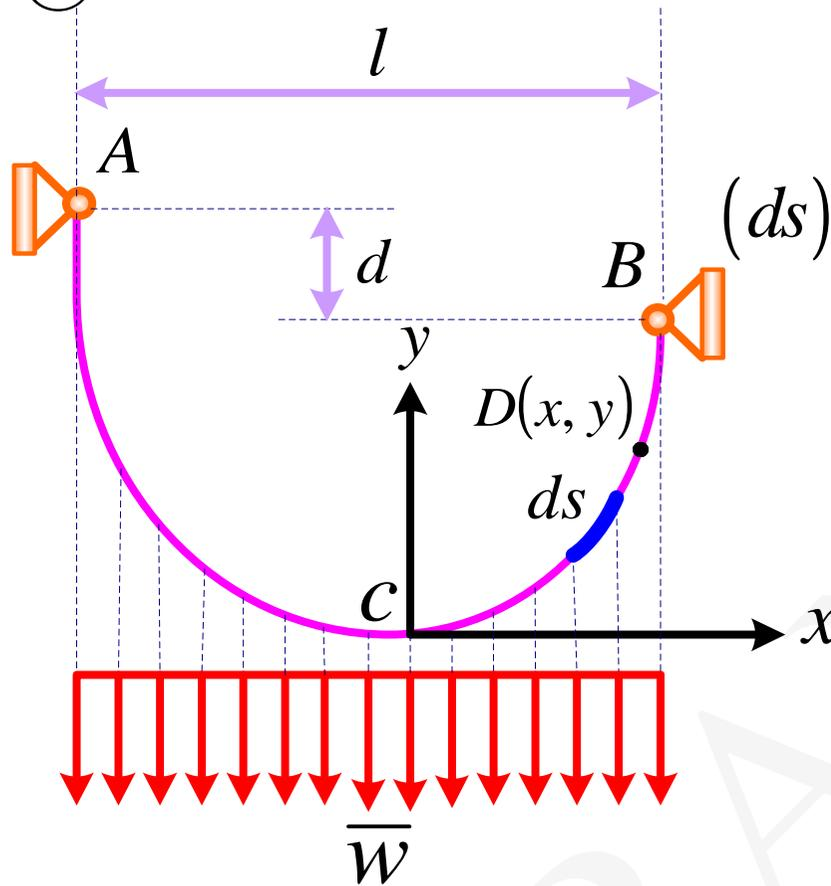
$$(ds)^2 = (dx)^2 + (dy)^2 = (dx)^2 \left[ 1 + \left( \frac{dy}{dx} \right)^2 \right]$$
