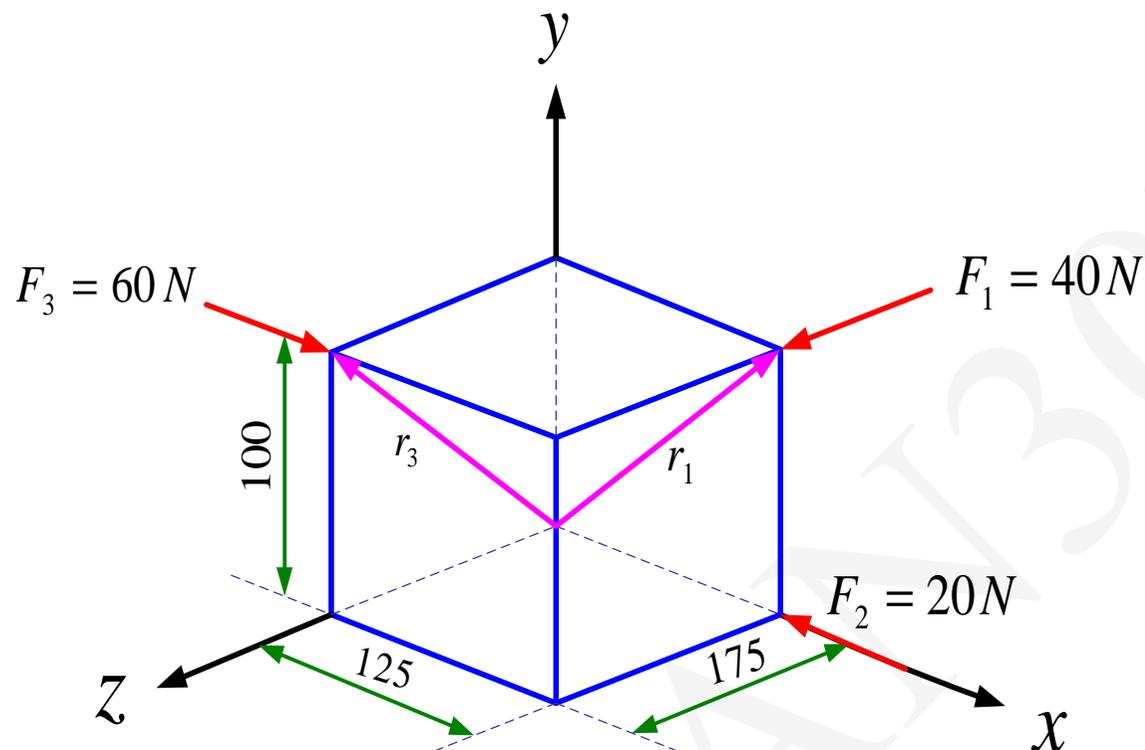
$$\underline{F}_1 = 40 \underline{k} \quad \underline{F}_2 = -20 \underline{i} \quad \underline{F}_3 = 60 \underline{i}$$
