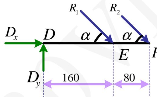
$$\sum M_D = 0 \Rightarrow R_1 \sin \alpha(0.16) + R_2 \sin \alpha(0.24) = 0 \quad \boxed{2R_1 + 3R_2 = 0}$$
