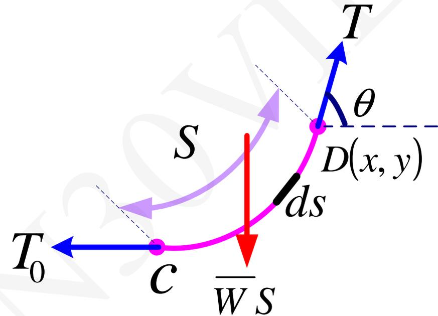
$$(ds)^2 = (dx)^2 + (dy)^2 = (dx)^2 \left[ 1 + \left( \frac{dy}{dx} \right)^2 \right] \quad \frac{dy}{dx} = \frac{\bar{W}S}{T_0}$$
