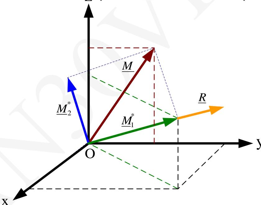
$$\underline{M} = \underline{M}_1^* + \underline{M}_2^* \quad \underline{\lambda}_R = \frac{\underline{R}}{R} = \frac{F_1 \underline{i} + F_2 \underline{j} + F_3 \underline{k}}{\sqrt{F_1^2 + F_2^2 + F_3^2}}$$
