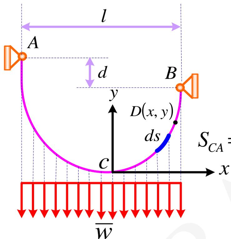
$$y_A = \frac{\bar{W}}{2T_0} x_A^2 \quad \frac{\bar{W}}{T_0} = 2 \frac{y_A}{x_A^2}$$
