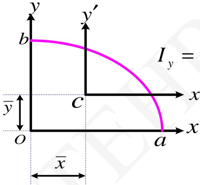
$$I_y = I_{y'} + A\bar{x}^2 \Rightarrow \frac{\pi ba^3}{16} = I_{y'} + \frac{\pi ab}{4} \left( \frac{16a^2}{9\pi^2} \right)$$
