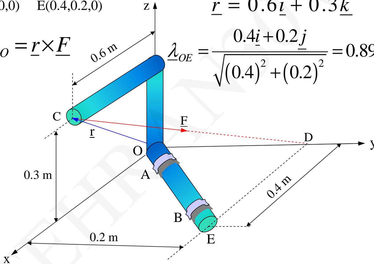
$$M_{AB} = \underline{\lambda}_{OE} \cdot \underline{M}_O = \underline{\lambda}_{OE} \cdot (\underline{r} \times \underline{F})$$
