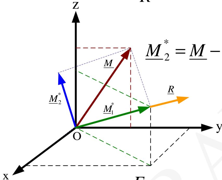
$$\underline{M}_2^* = \underline{M} - \underline{M}_1^* = cF_1 \underline{j} + aF_2 \underline{k} - \frac{F_2}{R^2} (cF_1 + aF_3) \underline{R}$$
