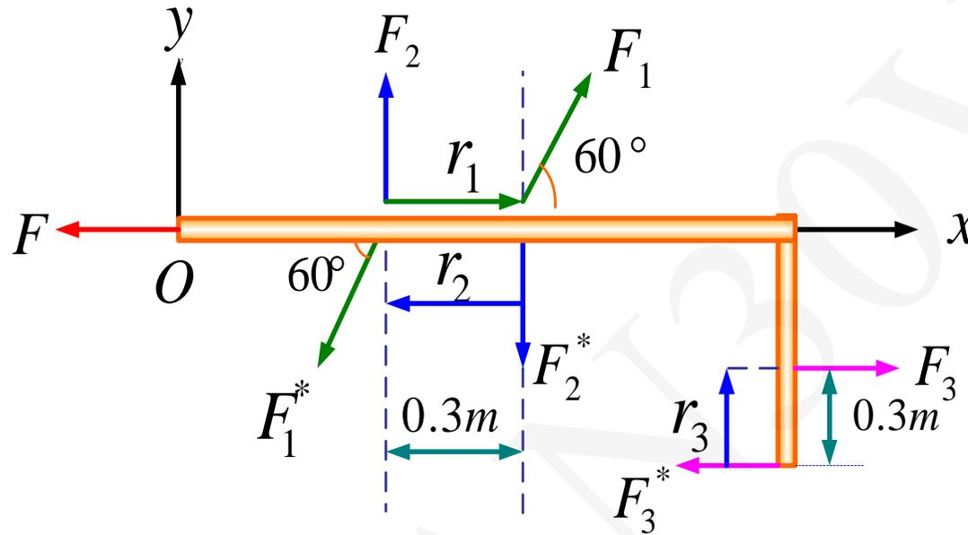
$$F = 200N \quad F_1 = F_1^* = 700N \quad F_2 = F_2^* = 500N \quad F_3 = F_3^* = 400N$$
