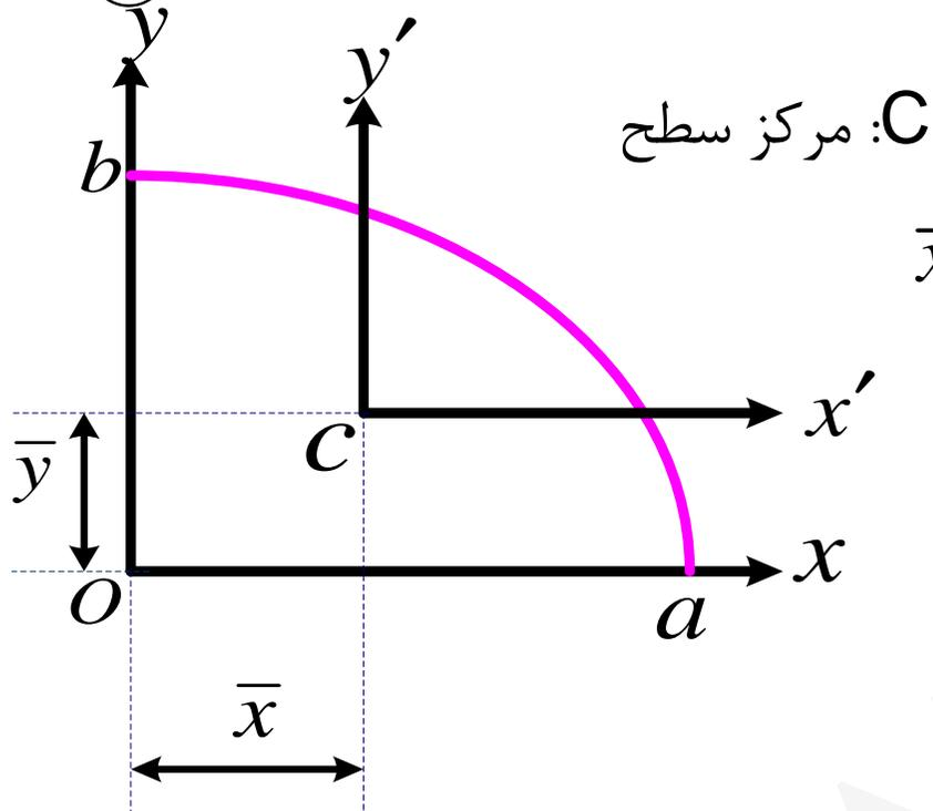
$$\bar{x} = \frac{\int \bar{x}_{el} dA}{A}, \quad \bar{y} = \frac{\int \bar{y}_{el} dA}{A}$$
