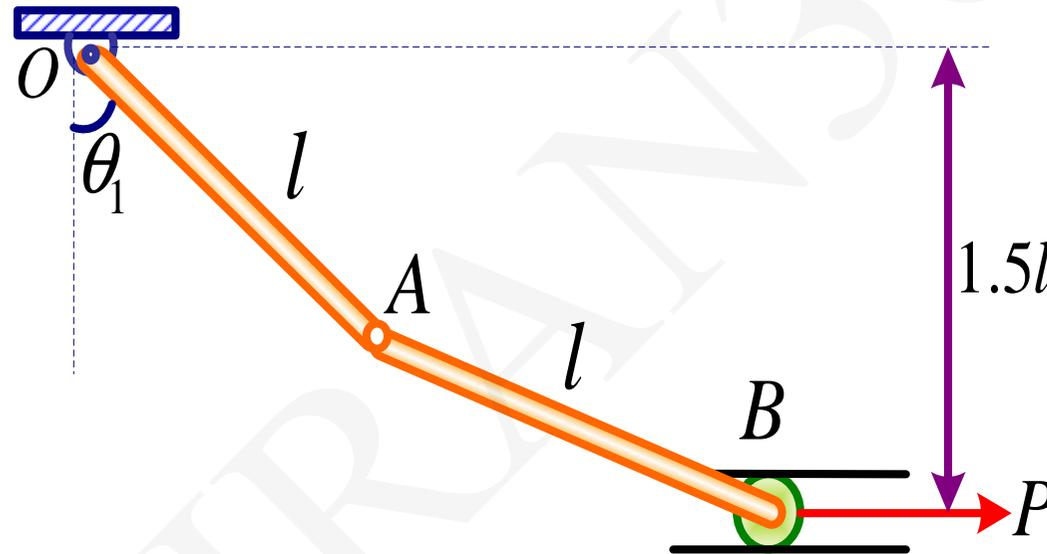
$$\delta U = \underline{w} \cdot \delta \underline{y}_{-1} + \underline{w} \cdot \delta \underline{y}_{-2} + \underline{P} \cdot \delta \underline{x}_B$$
